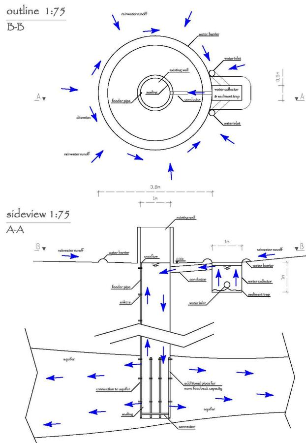
The solution is more than sustainable. It is a selfsufficient and sustainable reclamation utility that does not even require significant maintenance - just like a tree. It could be compared to a Palm Oasis because a large surface area receives a rainwater management system. The difference being that water is stored securely underground and the system is fully up and operational from the first rain event on.
